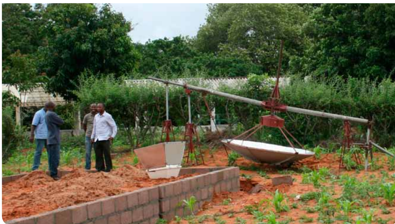
ENERGY GAIN: Four PhD students from the project Small Scale Solar Energy Systems, here standing in front of two solar energy prototypes at the Eduardo Mondlane University (UEM) Campus in Mozambique. UEM is cooperating with the Norwegian University of Science and Technology (NTNU) in this project. The small box is a solar cooker, whereas the large construction is a heat collector. "The sunbeams are reflected from the small mirrors to the receiver, which contains absorbing material. The absorbing material transforms the sunbeams into heat. In this construction (the pipe) the heat will be transported by air from the receiver to the storage. Now we are testing how much energy we can gain from this construction," explains PhD student Amos Veremachi.
